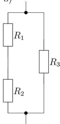
$$R_{\text{ges}} = (R_1 + R_2) \parallel R_3$$
