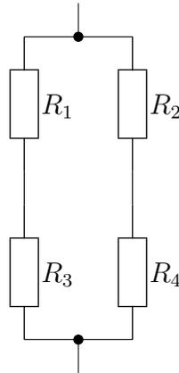
$$R_{\text{ges}} = (R_1 + R_3) \parallel (R_2 + R_4)$$
